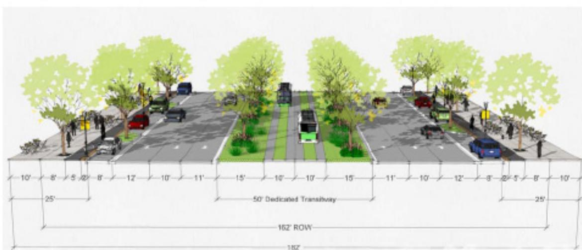
Figure 2: Alternative Rockville Pike BRT Cross Section
